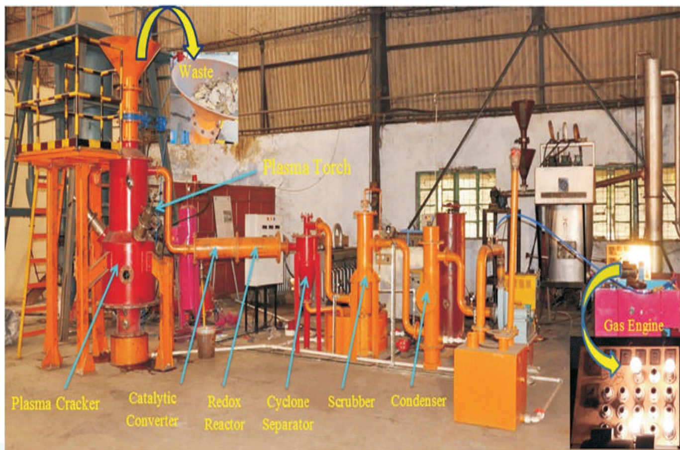
A 25 kg/h mini plant developed at CSIR-CMERI for eco friendly disposal of Municipal Solid Waste utilizing high temperature plasma
