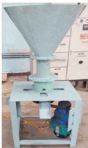
Figure 7: Biomass briquette making machine (left and middle) and its output
