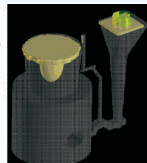
Figure 4: Solidification simulation of Al piston
