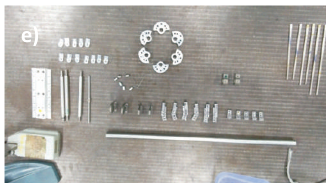
Figure 2: a) All Terrain Robot, b) Robotic Wheel Chair, c) Nozzle of MMD, d) Components of actuator, e) Components of fish-fin like bio-mimetic actuator, f) Hybrid fin of AUV 500.
