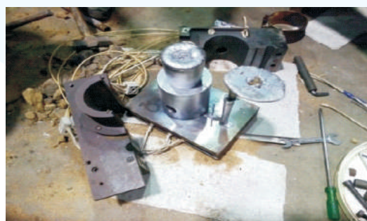
Figure 5: Cast blank of Al piston on the base of permanent mould
