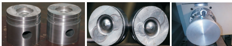
Figure 6: Photographs of machined surfaces of cast heat treated prototype Al piston developed at CSIR-CMERI
