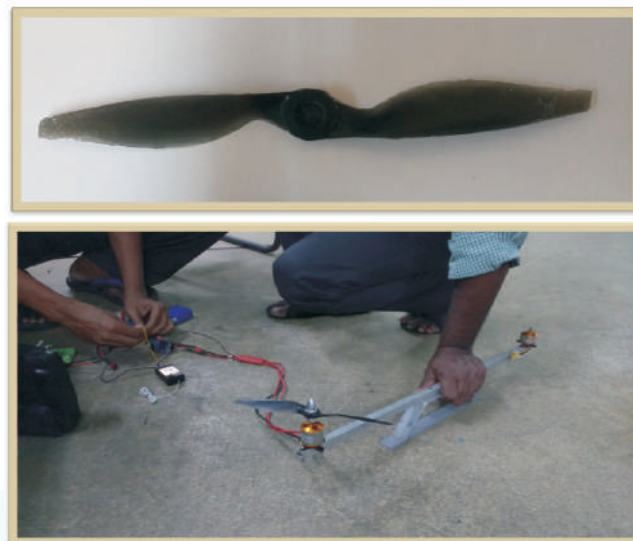
Figure 3: Developed drone blade using CNT reinforced epoxy composites
