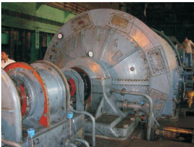
Vibration Analysis & in-situ balancing of Turbine Generator Set at PTPS, JSEB
