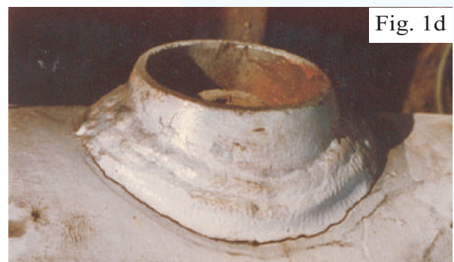
Figure 1d: Crack on Boiler Superheater Header
