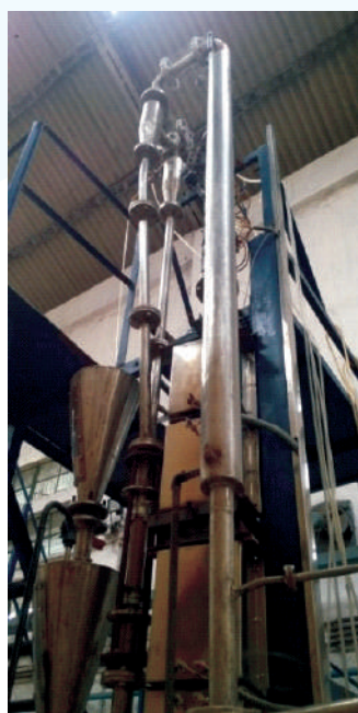
Figure 2: Experimental setup of laboratory scale circulating fluidized bed gasifier
