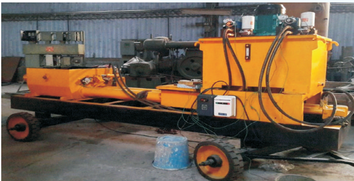
Figure 5: Lab Scale System for Transporting & Discharging of Viscous Semi Solid Material
