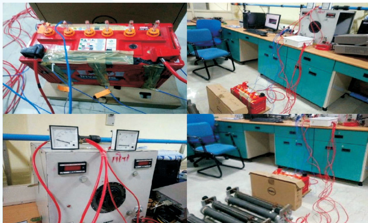
Experimental facility for battery performance testing using passive cooling medium
