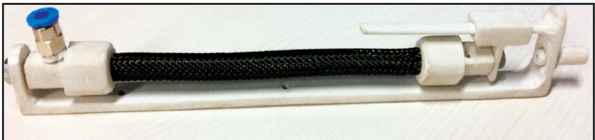
A version of indigenously developed light weight PAM actuator with 6 mm ID
