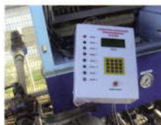
Figure Scheduler connected to irrigation & fertigation systems
