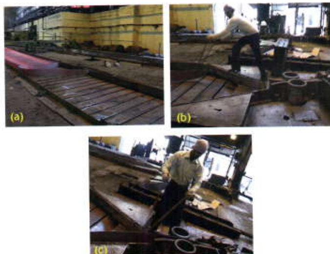
Figure 1: Present method of hot skelp coil tip feeding in-between CPR (a) Hot skelp on conveyor bed (b) Operator grasping the hot skelp with a tong (c) Operator feeding the hot skelp in-between CPR
