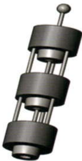
Figure 2: Solid Model of SMA actuated segments.
