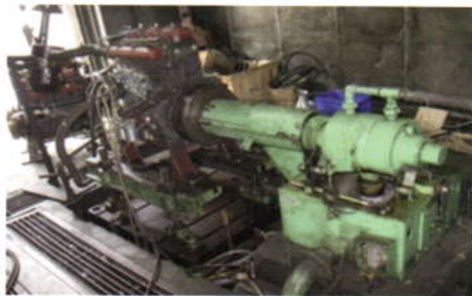
Figure 8: Photograph of 35 hp tractor engine being tested at ITL Hoshiarpur
