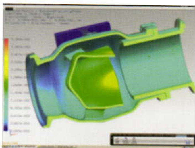
Figure 8: Axial sectional view of deformed valve body.
