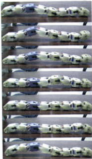
Figure 10: Caterpillar Rectilinear gait sequence
