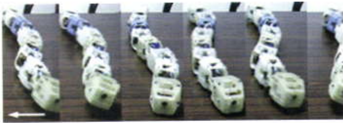
Figure 9: Frames showing gait sequence of Sidewinding locomotion. Frames are not necessarily at regular interval.
