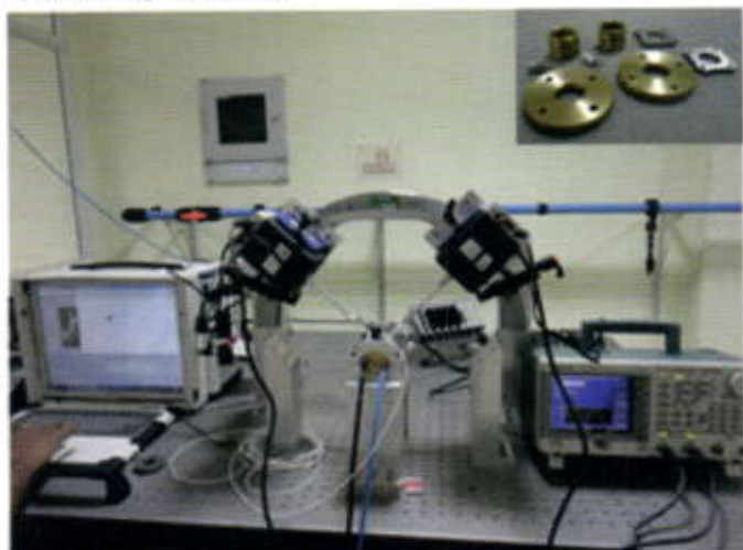
Innovative Gas Bearing Test Rig for directly evaluating dynamic coefficients of bearings
