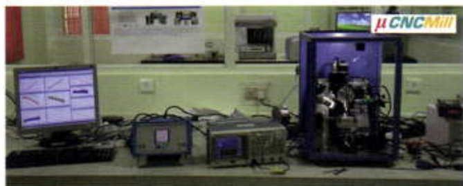
Five Axis \mu Milling Machine designed and developed by this group, First its kind in India.
