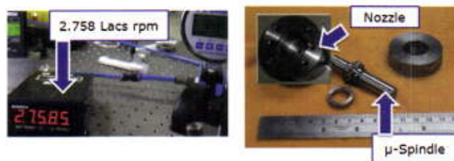
Demonstrated Microturbine running at 275000 rpm
