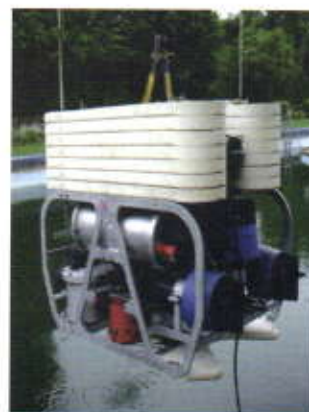
Figure 1: ROV-500 prototype equipped with thrusters, navigational & payload sensors
