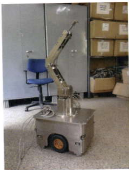
Figure 2: Robotic System – Vehicle with Manipulator
