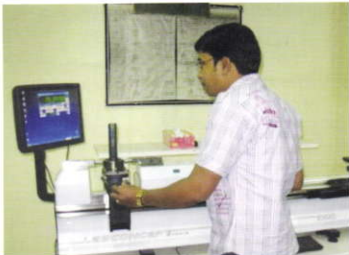
Figure 3: -Thread gauge calibration in Labconcept
