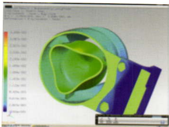
Figure 7: Transverse sectional view of deformed valve body.
