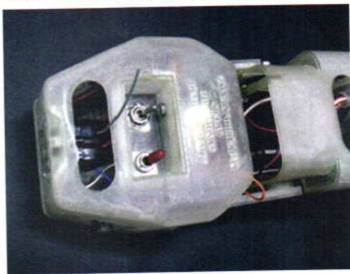
Figure 5: Video transmitter attached to the camera housed inside the head
