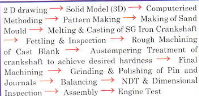
Figure 3: Flow chart for development of ADI Crankshaft
