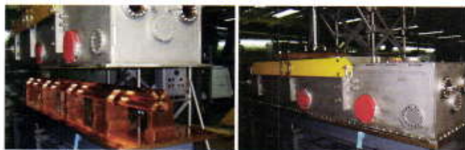
Figure -3: 40kW RFQ Cavity opened and closed.
