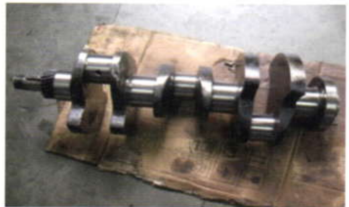
Figure 9: Photograph showing ADI crankshaft after 500hrs engine test
