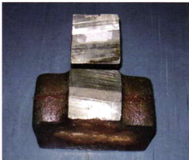
Figure 10: Photograph of cut section of neck area of cast swing hammer
