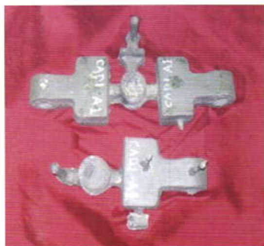
Figure 9: Photograph of cast hammers with side risers
