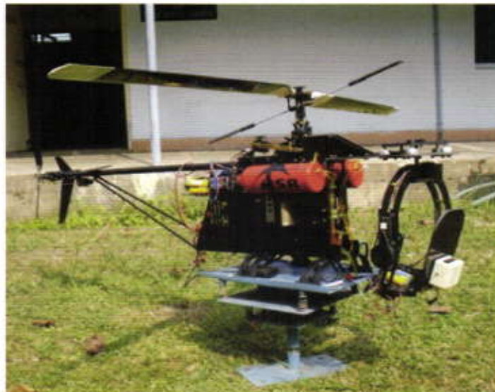
Rotorcraft Bergen Turbine Observer on a test rig for experimental data collection
