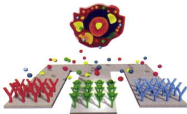
Fig 1: Proteins produced by cancer cells can be detected quickly using a cantilever device coated with specific antigens. When the proteins bind with the antigens, it changes the cantilever's oscillation rate
