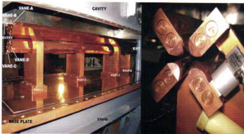
Experimental Setup for testing the modal response of RFQ Linac
