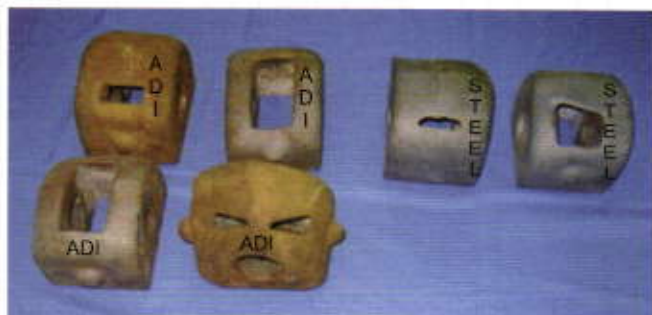
Figure 5: ADI and Steel beaer heads after 430 hours of operation
