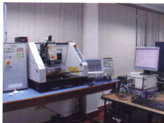
Fig 4: Micro Electric Discharge Machining Machine prototype developed at CMERI
