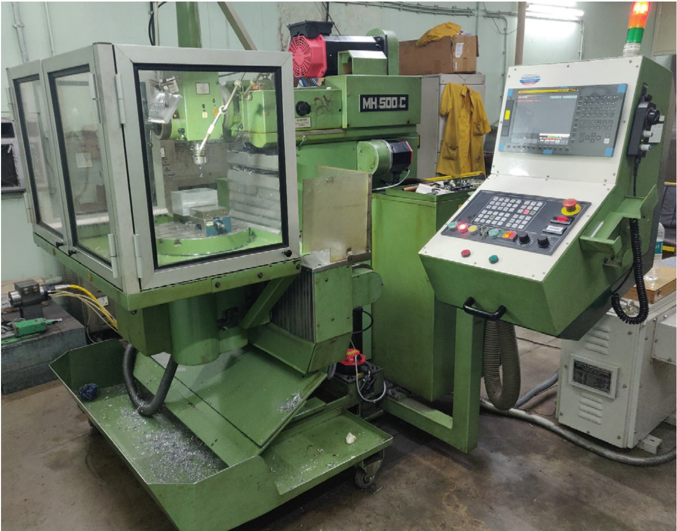
Images showing the retrofitted CNC MAHO 500C milling machine post installation and Commissioning
