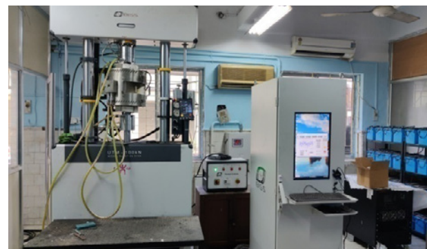
100kN UTM with High Temperature facility
