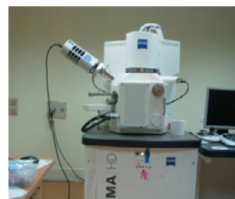
FESEM with attached EDS and Deformation stage
