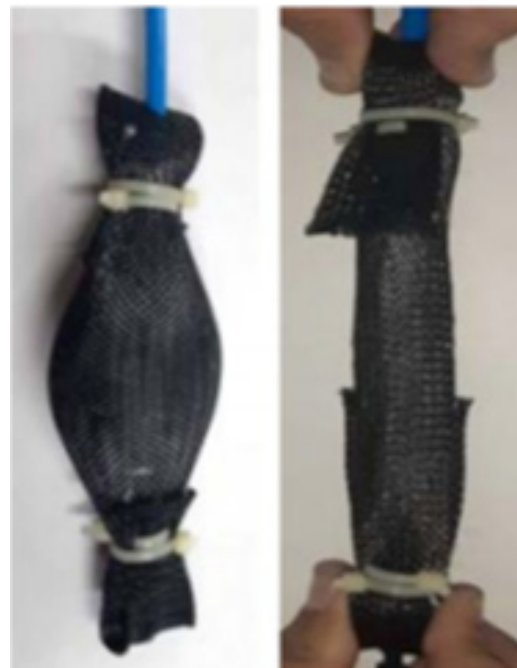
Fig.7 Low pressure Pneumatic Artificial Muscle (PAM) developed by CSIR-CMERI using hyper elastic silicone, intended for actuation of UAV manipulator.
