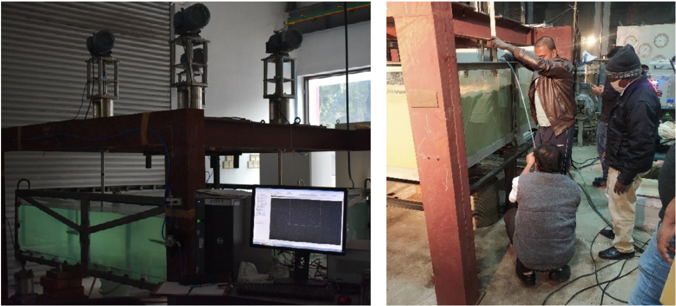
Fig. 3(a) Scaled down model of FGD plant (b) Collection of samples for measuring gypsum concentration in the slurry.
