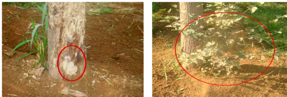
Fig.4: View of plant damage due to rotavator shield contour and weed left after operation.
