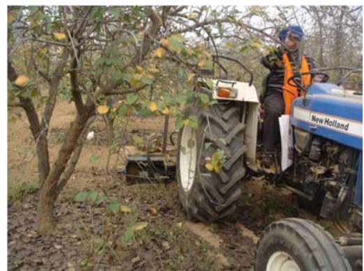
Fig.10: Limitation of offset rotavator in case of low height branching
