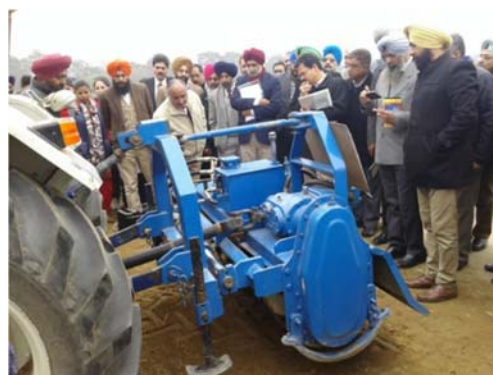
Fig.12: Demonstration of Offset rotavator to Extension Specialists of PAU and Deptt of Horticulture, Punjab
