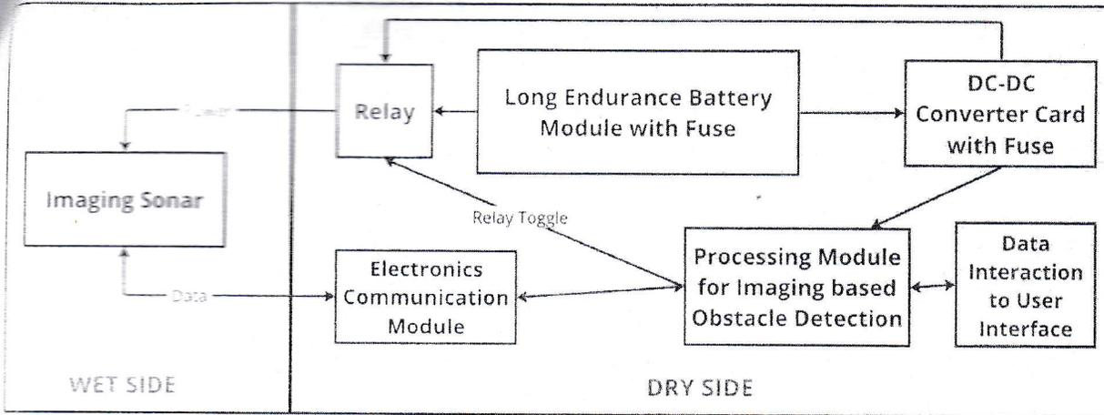
Supply of Customized Multi-Beam Long Endurance Forward Looking Sonar based System for Dynamic Obstacle Detection with an Underwater Robot as per design. Specifications of the Modules in the Design:
