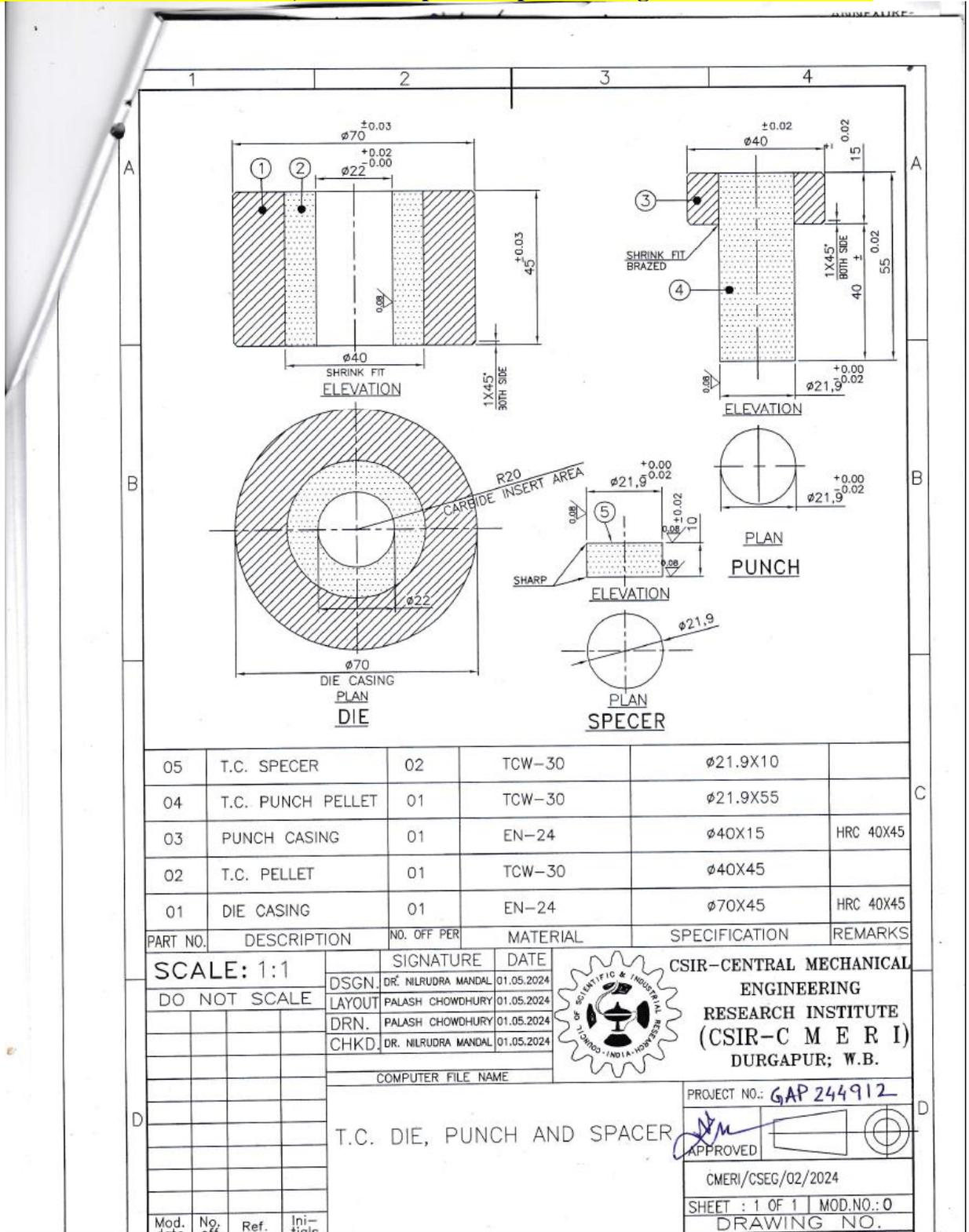
**3. Fabrication of Carbide Die, Punch & Spacer as per drawing no. CMERI/03/2024**
