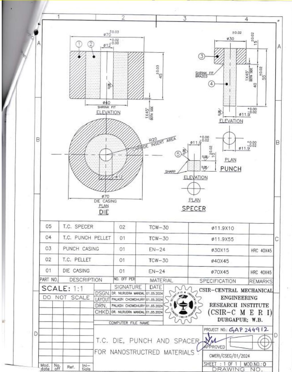
**2. Fabrication of Carbide Die, Punch & Spacer as per drawing no. CMERI/02/2024**
